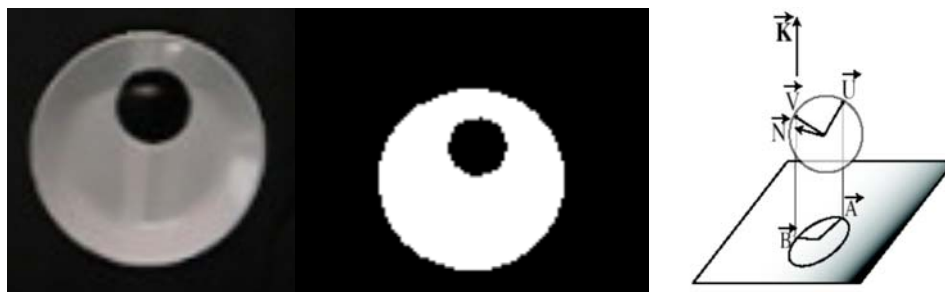
Figure 1: Video capture from plate experiment and reconstruction of its position
